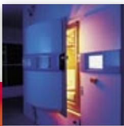
In ultra-modern vacuum coating facilities, a reflex-reducing layer is applied
